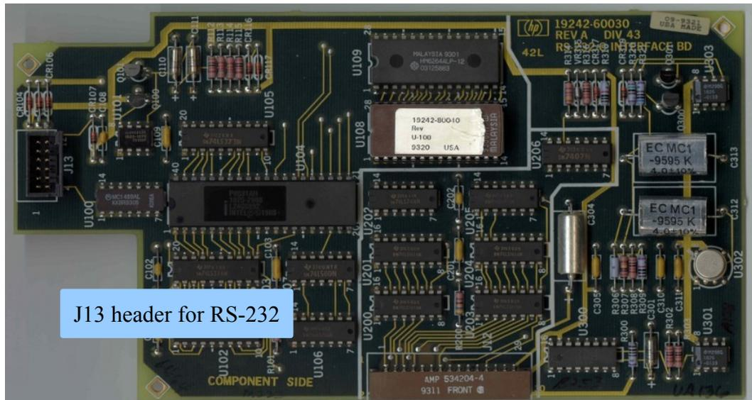
Fig. 1: 19242-xxxxx communication board connectors
